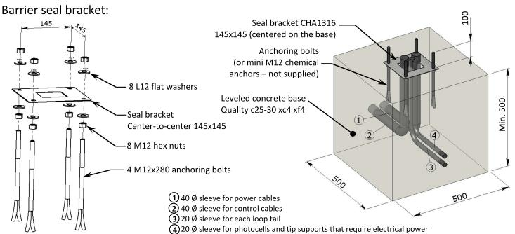
(Ensure the sleeves protrude 200mm)
